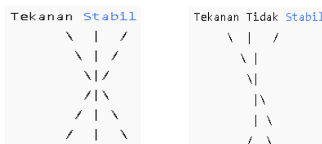
Figure 3. Comparison of Standard and Used Injector Spray Patterns
